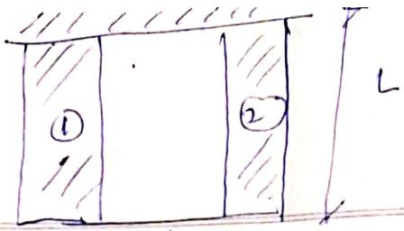
A composite bar is made of two or more bars of equal length but different materials rigidly fixed with each other and behaving as one unit for extension or compression when subjected to either tension or compression forces.
