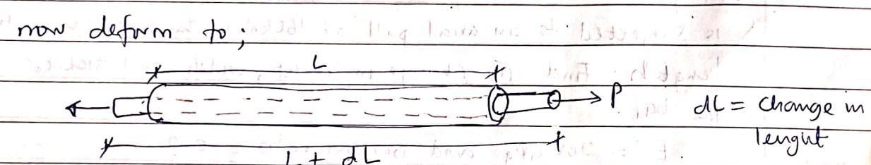
When there is a tensile force (pull) on a material, the length increases but the cross-sectional area of the material reduces (reduction in diameter).
